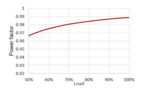
OT FIT 75 220-240 24 PC Typical Power Factor vs. Load
